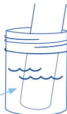
Bluelab pH Probe KCl Storage Solution
